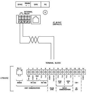
Verify Jumpers are "Open" as shown for Sync Output. To access jumpers see page 3.
